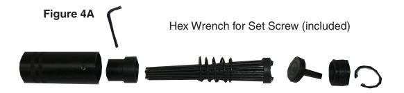
Insert the Needles (5A) through the holes in the Needle Holder (4A). There are nineteen Needles. Make sure all holes are filled before putting the Needle Holder (4A) through the Spring (3A), the Retainer Clip (2A) and into the Barrel Assembly (1A). Slide one Retainer Ring (8A) around the Needles (5A) and fasten it at the front end of the Barrel Assembly (1A). See Figures 4 & 4A
